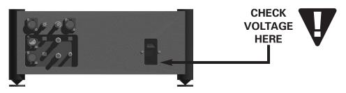
Check to make sure your Wadia S7i CD Player/Decoding Computer has been manufactured for operation at your AC line Voltage. Attempting to use the Player at any voltage other than the specified on the rear of the unit may damage the unit. Damage caused by improper operation is not covered by warranty. If the voltage specified is different from your AC voltage, contact your Wadia dealer.
