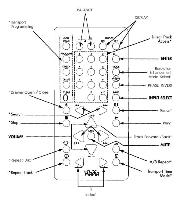
\* These buttons *are* used to control a Wadia Transport.
