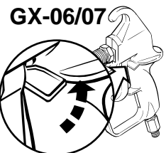
Gun locked (gun will not spray)
