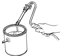
2. Remove paint in hose.
