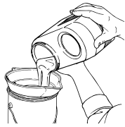
3. Empty fluid tank.
