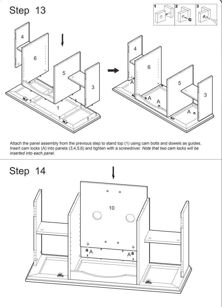
Carefully slide back panel (10) into place along the back of the stand assembly. Use cam bolts and dowels as guides. Insert cam locks (A) into back panel (10) and tighten with a screwdriver.
