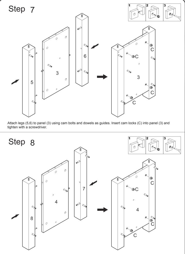
Attach legs (7,8) to panel (4) using cam bolts and dowels as guides. Insert cam locks (C) into panel (4) and tighten with a screwdriver.
