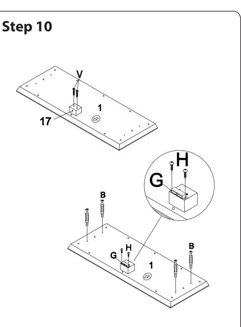
Attach block (17) to the stand top (1) using screws (V). Screw cam bolts (B) into stand top (1), then attach door stop (G) using screws (H) as shown in the diagram. *Be sure to tighten firmly.*
