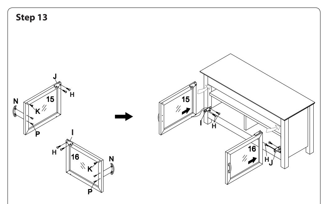
Attach door handles (N) to the stand doors (15,16) using screws (P). Attach screws (K) to the corners of each door as shown in the diagram. Attach hinge (J) to door (15) as shown in the diagram. Attach hinge (I) to door (16) as shown in the diagram. Insert lower door hinges (I, J) into the lower pivot points. Attach doors (15,16) to the stand at the upper pivot points as shown in the diagram. Attach doors to lower door hinges (I, J) using screws (H).
