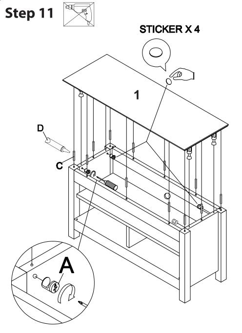
Insert dowels (C) into frame assembly. (*Remember to apply glue (D)*) Insert cam locks (A) into frame assembly. Attach stand top (1) to the frame assembly. Tighten cam locks (A) using a screwdriver as shown in the diagram. Place provided stickers over cam locks (A).
