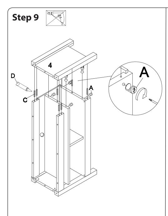
Insert dowels (C) into frame assembly (remember to apply glue (D)). Insert cam locks (A) into frame assembly. Attach right side assembly (4) to the frame assembly. Tighten cam locks (A) using a screwdriver as shown in the diagram.
