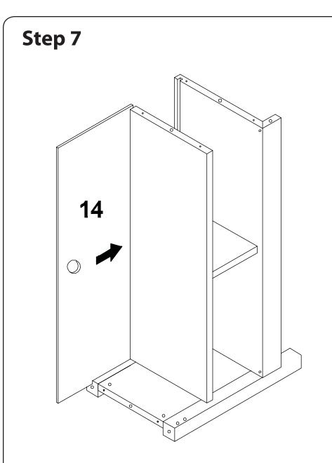
Slide back panel (14) into the grooves as shown in the diagram. Be sure that the side with the warning label is facing outward.
