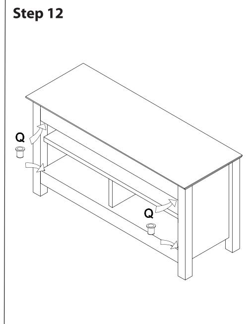
Insert the plastic pivots (Q) into the stand as shown in the diagram.
