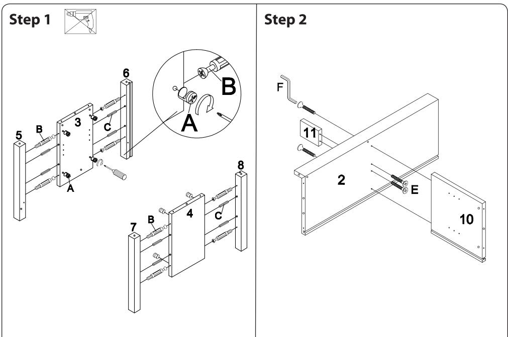
Insert dowels (C) and cam bolts (B) into side panels (3 & 4).
