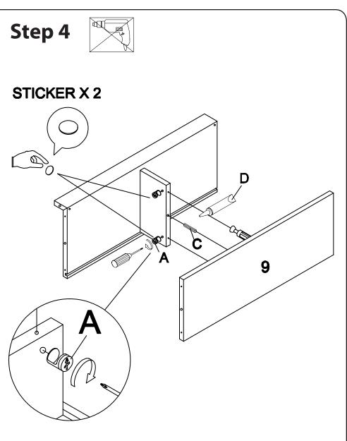
Insert dowels (C) into the left side panel (3). *(Remember to apply glue (D))* Insert cam locks (A) into frame assembly. Attach middle shelf (9) to frame assembly. Tighten cam locks (A) with a screwdrivers as shown in the diagram.
