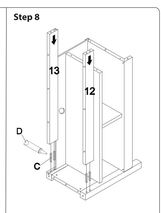
Insert dowels (C) into frame assembly. (*Remember to apply glue (D*)) Attach supports (12,13) to the frame assembly as shown in the diagram.
