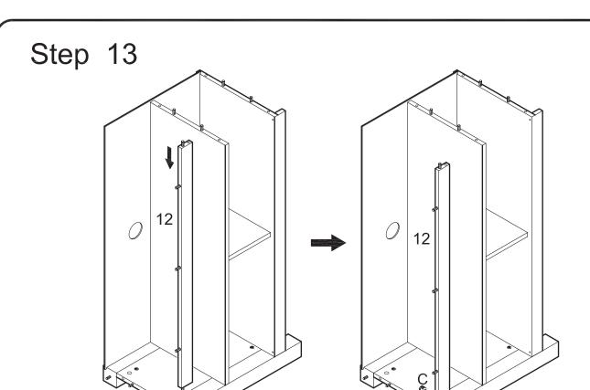
Attach slat (12) to the frame assembly using cam bolt and dowel as guides. Insert cam lock (C) into slat (12) and tighten with a screwdriver.
