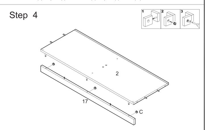
Attach slat (17) to panel (2) using cam bolts and dowels as guides. Insert cam locks (C) into slat (17) and tighten with a screwdriver.
