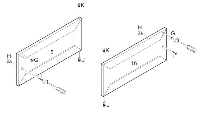
Attach handles (H) to doors (15,16) using medium bolts (I). Screw short bolts (G) into doors (15,16). Insert fixed door hinges (J) and spring door hinges (K) into doors (15,16).
