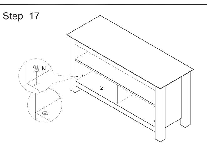
Insert plastic pivots (N) into panel (2).
