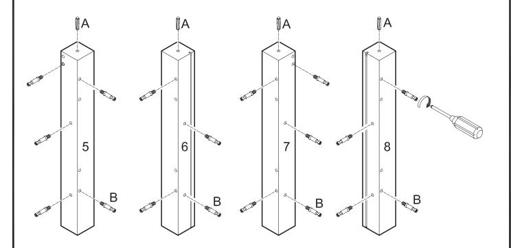
Screw cam bolts (B) into legs (5,6,7,8). Insert dowels (A) into legs (5,6,7,8).
