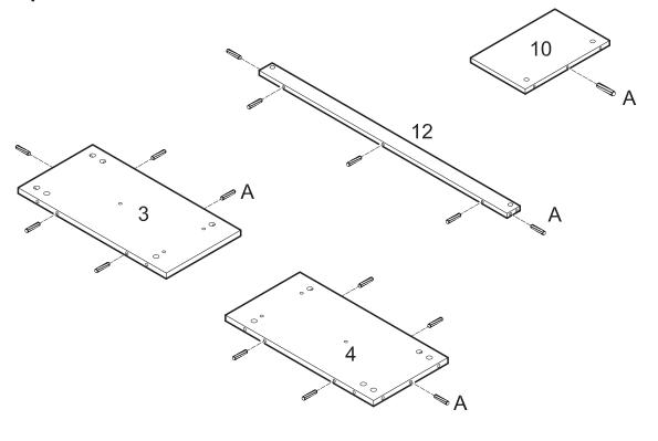
Insert dowels (A) into panels (3,4,10) and slat (12).
