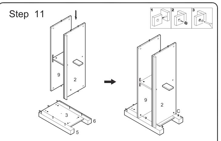
Attach the assembly from the previous step to the panel (3) assembly using cam bolts and dowels as guides. Insert cam locks (C) into panel (2) and shelf (9) and tighten with a screwdriver. Two cam locks will be inserted into panel (2) and into the shelf (9).
