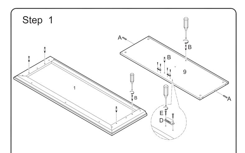
Screw cam bolts (B) into top panel (1) and shelf (9). Insert dowels (A) into shelf (9). Attach door stoppers (D) to shelf (9) using small screws (E).
