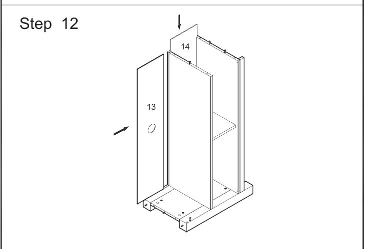
Carefully slide back panels (13,14) into place along the grooves at the back of the frame assembly.
