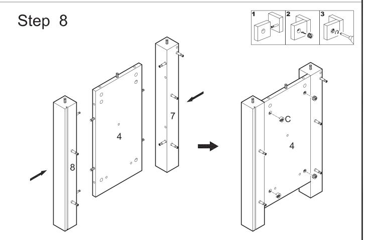
Attach legs (7,8) to panel (4) using cam bolts and dowels as guides. Insert cam locks (C) into panel (4) and tighten with a screwdriver.
