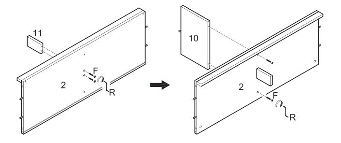
Attach support leg (11) to panel (2) using long bolts (F). Tighten long bolts (F) with wrench (R). Attach panel (10) to panel (2) using long bolts (F). Tighten long bolts (F) with wrench (R).
