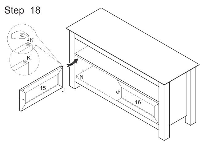
Attach door (15) to the stand by first inserting fixed door hinge (J) into plastic pivot (N). Depress spring door hinge (K) as you slide door (15) into place. Repeat this process for door (16).
