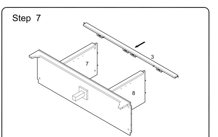
Attach slat (3) to the assembly from the previous step using dowels as a guide.
