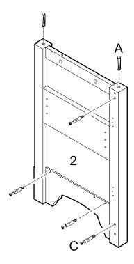
Insert large dowels (A) into side panels (1,2). Screw cam bolts (C) into side panels (1,2).
