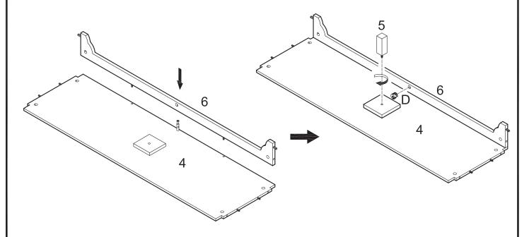
Attach slat (6) to bottom panel (4) using cam bolt and dowels as guides. Insert cam lock (D) into slat (6) and tighten with a screwdriver. Screw leg (5) into bottom panel (4).
