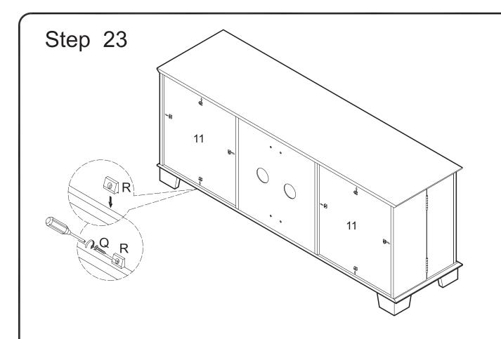
Secure back panels (11) using plastic wedges (R) and medium screws (Q).
