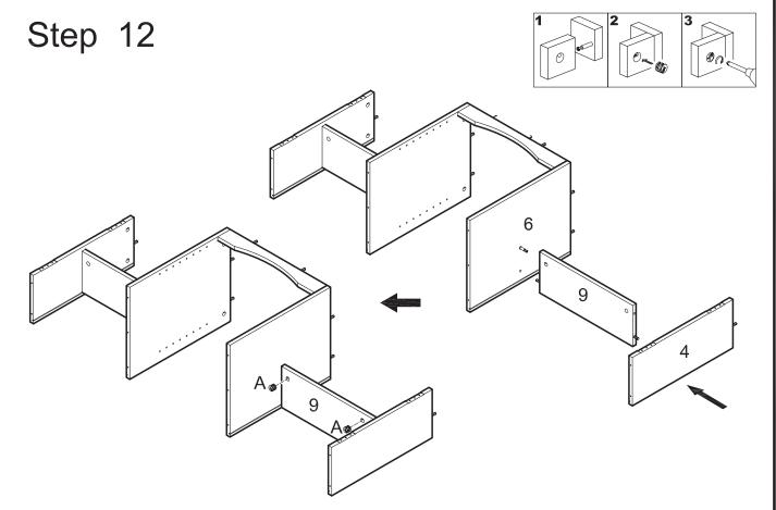
Attach shelf (9) to panel (6), then panel (4) to shelf (9) using cam bolts and dowels as guides. Insert cam locks (A) into shelf (9) and tighten with a screwdriver.
