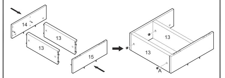
Attach panels (14,15) to shelves (13) using cam bolts and dowels as guides. Insert cam locks (A) into shelves (13) and tighten with a screwdriver. *Note that two cam locks will be inserted into each shelf.*
