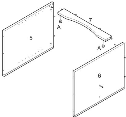
Insert cam locks (A) into slat (7). Attach panels (5,6) to slat (7) using cam bolts and dowels as guides. Tighten cam locks (A) with a screwdriver.
