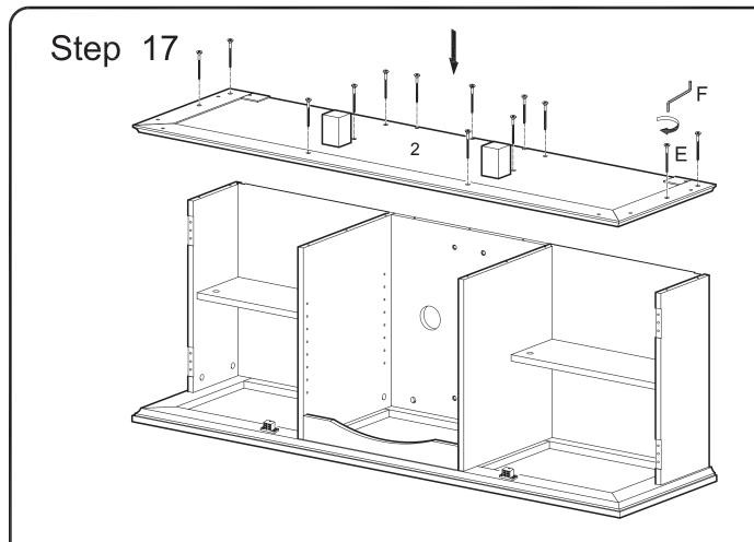
Attach stand base (2) to the stand assembly using bolts (E). Tighten bolts (E) with wrench (F).
