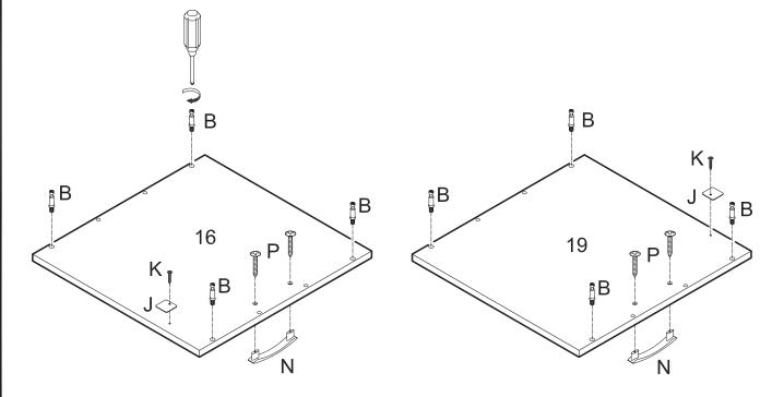
Screw cam bolts (B) into doors (16,19). Attach door stopper plates (J) to doors (16,19) using small screws (K). Attach handles (N) to doors (16,19) using large round head screws (P).
