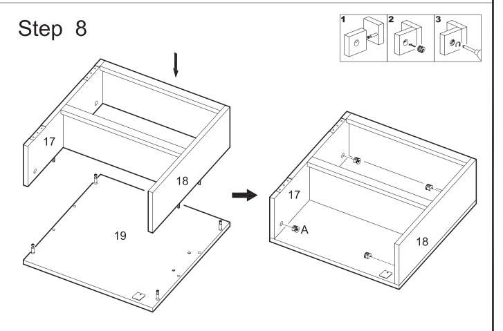
Attach the shelf assembly from the previous step to door (19) using cam bolts and dowels as guides. Insert cam locks (A) into panels (17,18) and tighten with a screwdriver.
