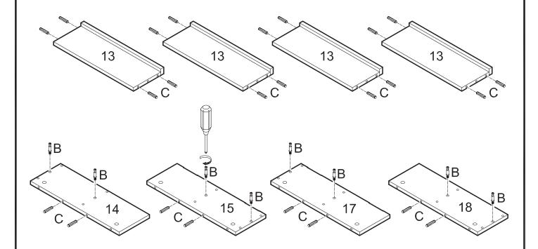
Insert dowels (C) into shelves (13) and panels (14,15,17,18). Screw cam bolts (B) into panels (14,15,17,18).
