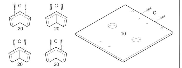
Insert dowels (C) into feet (20) and back panel (10).
