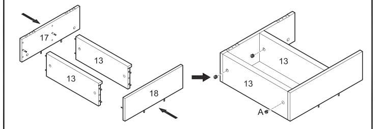
Attach panels (17,18) to the second set of shelves (13) using cam bolts and dowels as guides. Insert cam locks (A) into shelves (13) and tighten with a screwdriver. *Note that two cam locks will be inserted into each shelf.*
