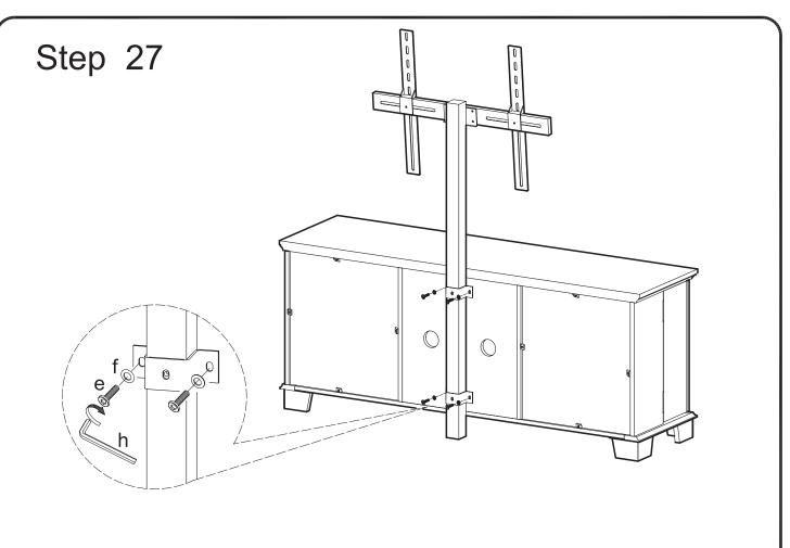
Attach TV mount to stand assembly using bolts (e) and washers (f). Tighten bolts (e) with wrench (h).
