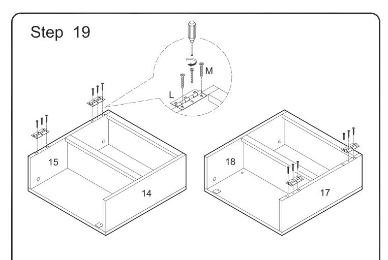
Attach door hinges (L) to the door assemblies from Steps 8 and 9 using large screws (M).
