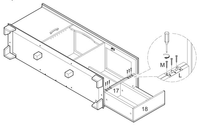
Attach door assembly (17,18) to the opposite side of the stand assembly at door hinges (L) using large screws (M).
