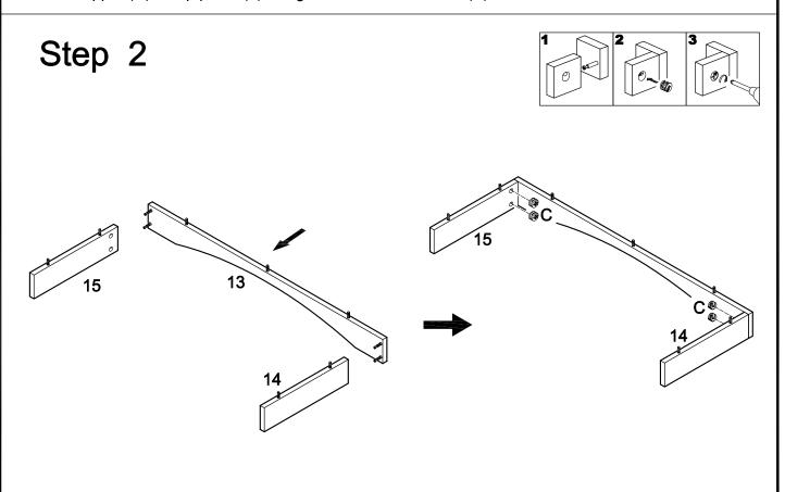
Attach slats (14,15) to slat (13) using cam bolts as guides. Insert cam locks (C) into slats (14,15) and tighten with a screwdriver.
