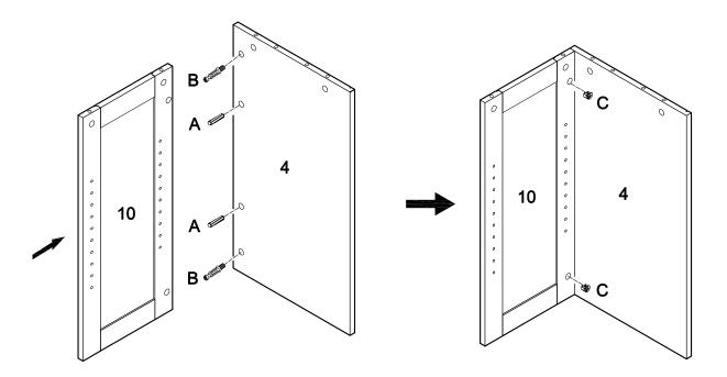
Screw cam bolts (B), and insert dowels (A) into panel (4). Attach panel (10) to panel (4) using cam bolts and dowels as guides. Insert cam locks (C) into panel (10) and tighten with a screwdriver.
