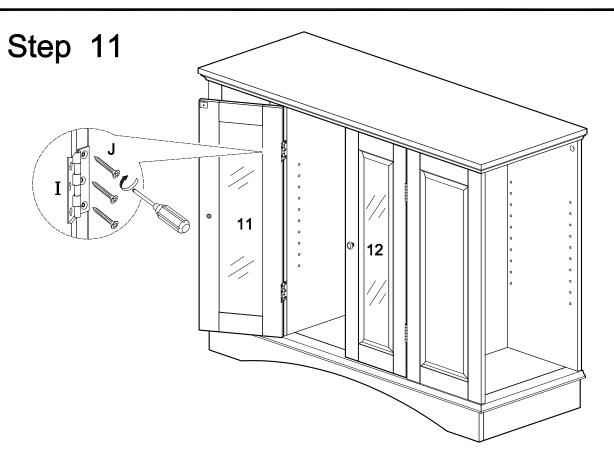
Attach doors (11,12) to the stand assembly at hinges (I) using medium screws (J). For proper alignment of doors, it may be necessary to loosen small screws (J), adjust the placement of hinges (I) and re-tighten screws (J).
