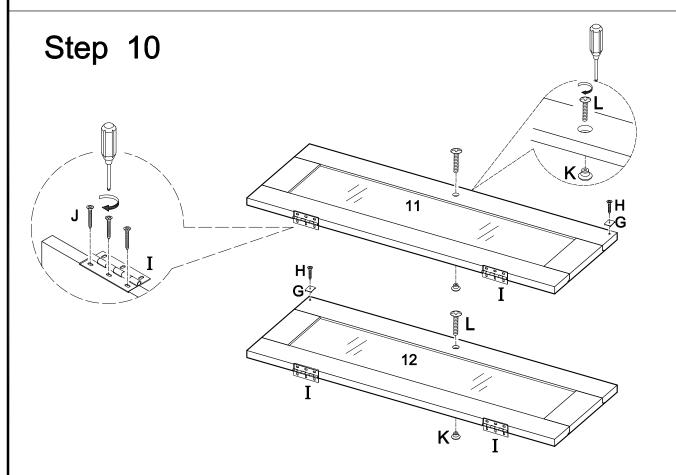
Attach door hinges (I) to doors (11,12) using medium screws (J). Attach handles (K) to doors (11,12) using small bolts (L). Attach door stopper plates (G) to doors (11,12) using small screws (H).
