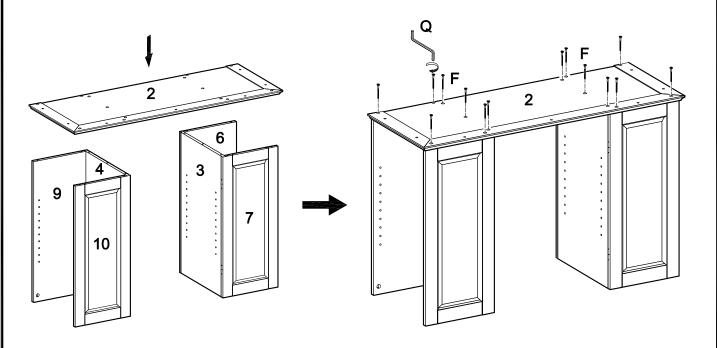
Attach bottom panel (2) to the panel assemblies from Steps 3 and 4, and to panels (6,9) using large bolts (F) and wrench (Q). Note that panels (6,9) will not be directly attached to the panel assemblies from Steps 3 and 4.
