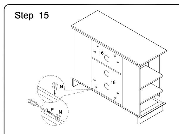
Secure back panels (16,18) using plastic wedges (N) and large screws (P).
