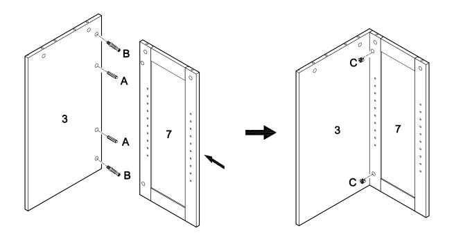
Screw cam bolts (B), and insert dowels (A) into panel (3). Attach panel (7) to panel (3) using cam bolts and dowels as guides. Insert cam locks (C) into panel (7) and tighten with a screwdriver.
