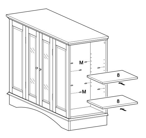
Insert shelf support pins (M) into the stand at desired shelf heights. Carefully place shelves (8) onto shelf support pins (M). Note that there will be two shelf support pins (M) on either end of each shelf (8).
