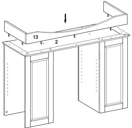
Attach the base assembly from Step 2 to bottom panel (2) by inserting the dowels of the base assembly into the pre-drilled holes of bottom panel (2).
