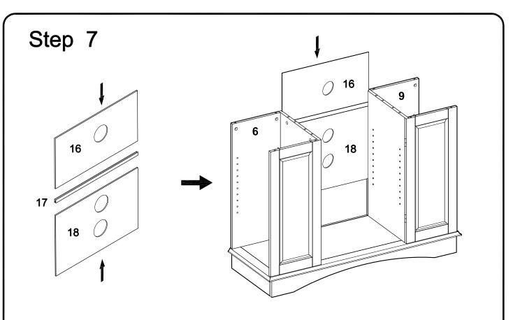
Slide back panel (18), back slat (17) then back panel (16) into the stand assembly.
