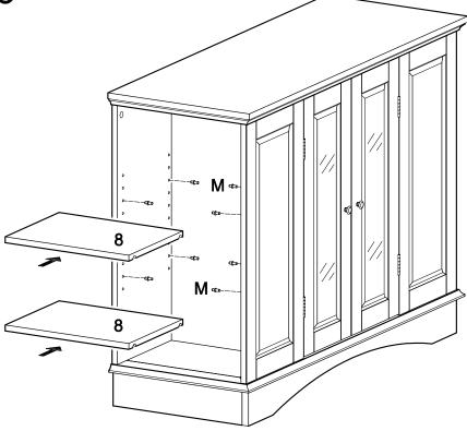
Insert shelf support pins (M) into the stand at desired shelf heights. Carefully place shelves (8) onto shelf support pins (M). Note that there will be two shelf support pins (M) on either end of each shelf (8).
