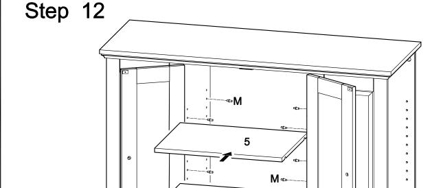
Insert shelf support pins (M) into the stand at desired shelf heights. Carefully place shelves (5) onto shelf support pins (M). Note that there will be two shelf support pins (M) on either end of each shelf (5).
