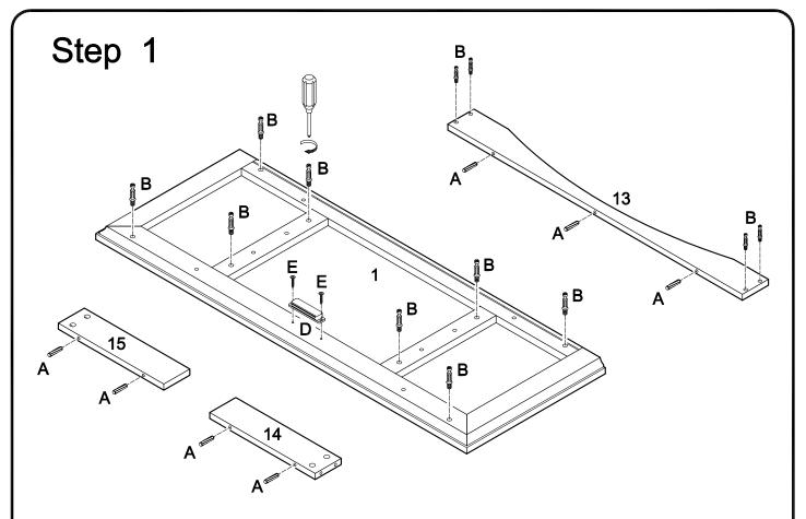
Insert dowels (A) into slats (13,14,15). Screw cam bolts (B) into top panel (1) and slat (13). Attach door stopper (D) to top panel (1) using round-headed screws (E).
