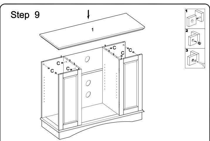
Insert cam locks (C) into the stand assembly. Attach top panel (1) to the stand assembly using cam bolts and dowels as guides. Tighten cam locks (C) with a screwdriver to secure top panel (1).
