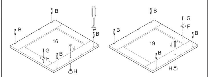
Screw cam bolts (B) into panels (16,19). Attach handles (H) to panels (16,19) using small bolts (J). Attach door stopper plates (F) to panels (16,19) using small screws (G).
