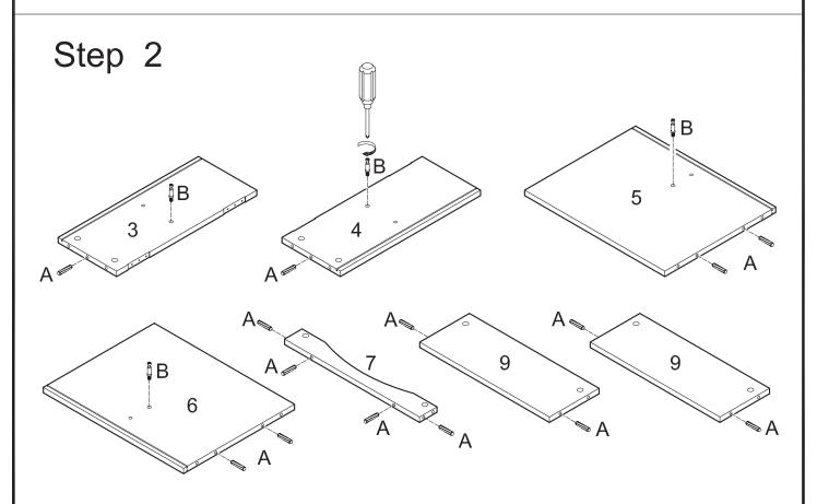
Screw cam bolts (B) into panels (3,4,5,6). Insert dowels (A) into panels (3,4,5,6), slat (7) and shelves (9).
