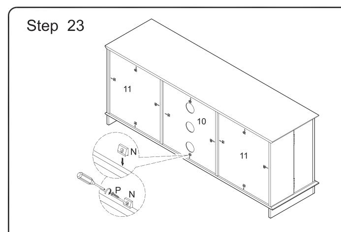
Secure back panels (10,11) using plastic wedges (N) and large screws (P).
