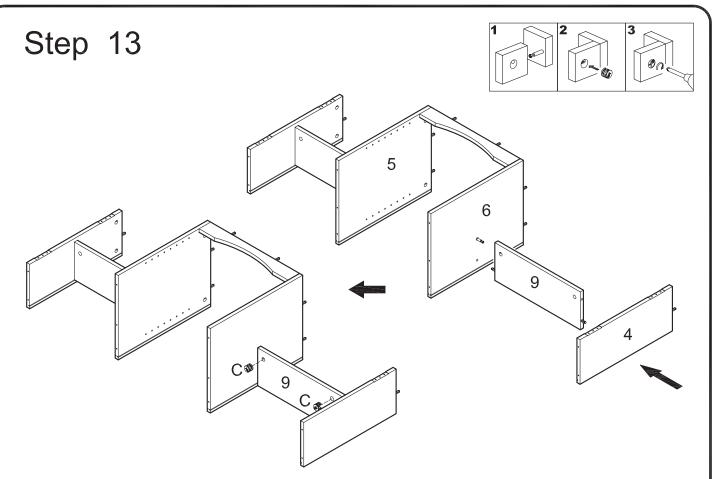
Attach shelf (9) to the panel (5,6) assembly, then attach panel (4) to shelf (9) using cam bolts and dowels as guides. Insert cam locks (C) into shelf (9) and tighten with a screwdriver.
