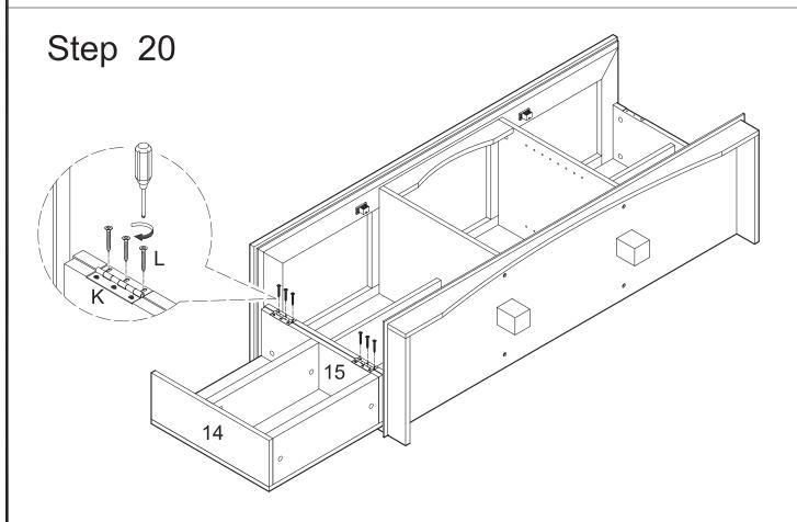
Attach the panel (14,15) assembly to the stand assembly at door hinges (K) using extra-large screws (L).
