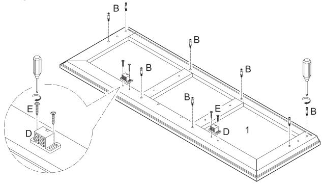
Screw cam bolts (B) into stand top (1). Attach door stoppers (D) to stand top (1) using medium screws (E).
