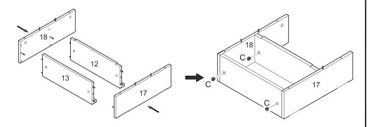
Attach panels (17,18) to shelves (12,13) using cam bolts and dowels as guides. Insert cam locks (C) into shelves (12,13) and tighten with a screwdriver. Note that two cam locks (C) will be inserted into each shelf (12,13).
