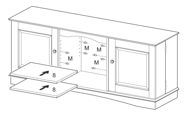
Insert shelf support pins (M) into the stand assembly at desired shelf heights. Carefully place shelves (8) onto shelf support pins (M). Note that there will be two shelf support pins (M) on either end of each shelf (8).
