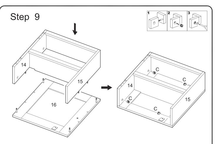
Attach the panel (14,15) assembly to panel (16) using cam bolts and dowels as guides. Insert cam locks (C) into panels (14,15) and tighten with a screwdriver.
