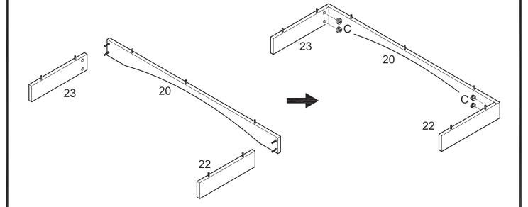
Attach slats (22,23) to slat (20) using cam bolts as guides. Insert cam locks (C) into slats (22,23) and tighten with a screwdriver.
