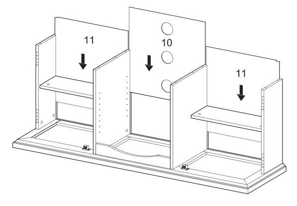
Slide back panels (10,11) into the appropriate grooves at the back of the stand assembly.
