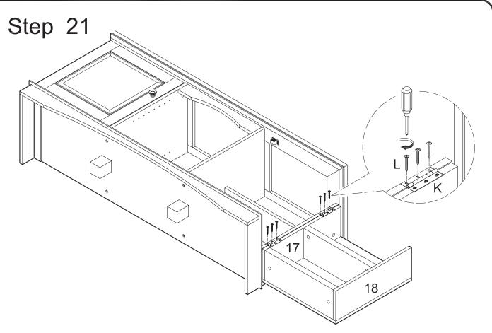
Attach the panel (17,18) assembly to the stand assembly at door hinges (K) using extra-large screws (L).
