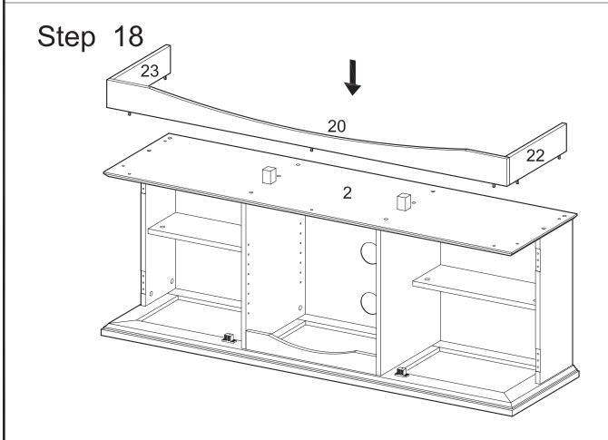
Attach the slat (20,22,23) assembly to stand base (2) using cam bolts and dowels as guides.
