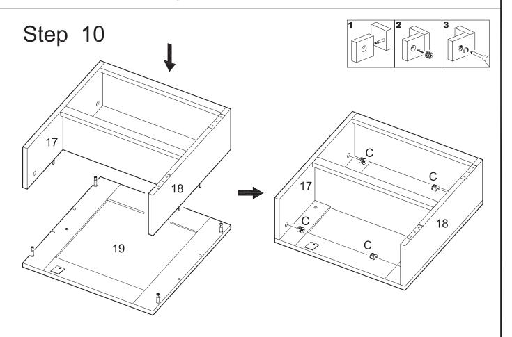
Attach the panel (17,18) assembly to panel (19) using cam bolts and dowels as guides. Insert cam locks (C) into panels (17,18) and tighten with a screwdriver.
