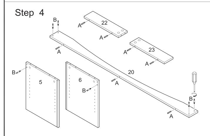
Screw cam bolts (B) into panels (5,6) and slat (20). Insert dowels (A) into slats (20,22,23).
