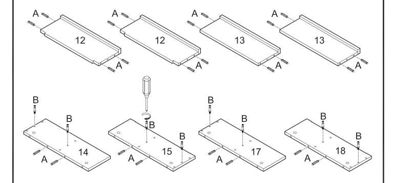
Screw cam bolts (B) into panels (14,15,17,18). Insert dowels (A) into panels (14,15,17,18) and shelves (12,13).
