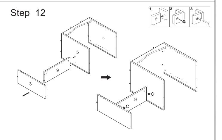
Attach shelf (9) to the panel (5,6) assembly, then attach panel (3) to shelf (9) using cam bolts and dowels as guides. Insert cam locks (C) into shelf (9) and tighten with a screwdriver.
