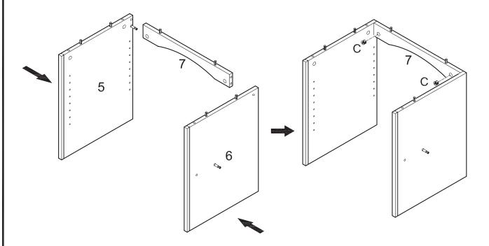
Attach panels (5,6) to slat (7) using cam bolts and dowels as guides. Insert cam locks (C) into slat (7) and tighten with a screwdriver.
