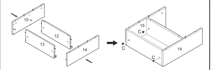
Attach panels (14,15) to shelves (12,13) using cam bolts and dowels as guides. Insert cam locks (C) into shelves (12,13) and tighten with a screwdriver. Note that two cam locks (C) will be inserted into each shelf (12,13).
