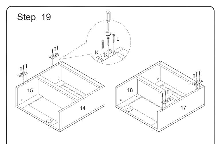
Attach door hinges (K) to panels (15,17) using extra-large screws (L).
