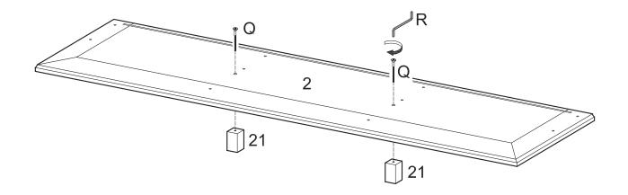
Attach feet (21) to stand base (2) using large bolts (Q) and wrench (R).
