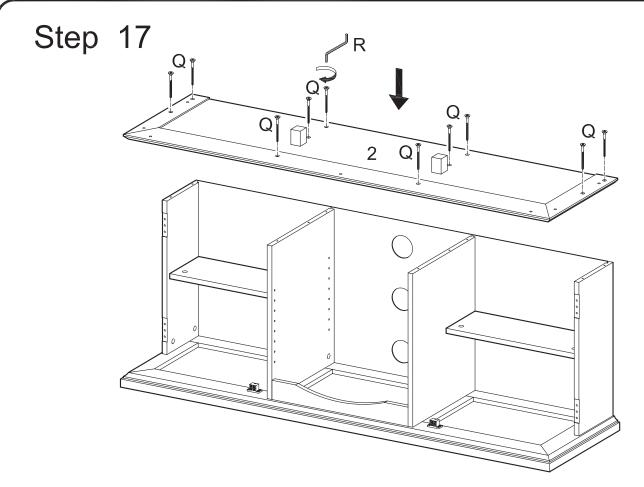
Attach stand base (2) to the stand assembly using large bolts (Q) and wrench (R).
