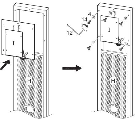
Attach pivoting bracket (I) to upper cable management system (H) using bolts (14) and washers (4). Tighten bolts (14) with wrench (12).
