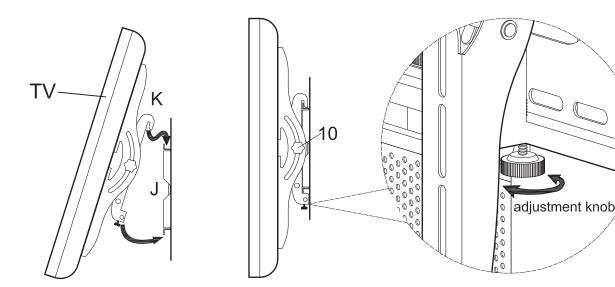
Loosen the adjustment knobs at the base of mounting brackets (K). Carefully hook mounting brackets (K) onto base bracket (J). Tighten the adjustment knobs at the base of mounting brackets (K) to secure the TV to the mount. To adjust the tilt of the TV, loosen tilt adjustment knobs (10), tilt TV up or down then tighten tilt adjustment knobs (10).
