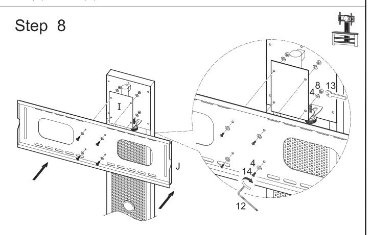
Attach base bracket (J) to pivoting bracket (I) by inserting bolts (14) with washers (4) through base bracket (J) and pivoting bracket (I) as shown above. Then, screw nuts (8) with washers (4) onto bolts (14). Using wrenches (12,13) together, firmly tighten bolts (14) and nuts (8).
