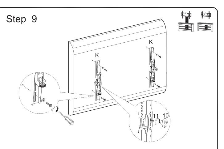
Attach mounting brackets (K) to the TV using the appropriate hardware from the TV mounting hardware kit. *Appropriate hardware will vary depending on TV type.* Attach tilt adjustment knobs (10) to mounting brackets (K) using flange bolts (11).
