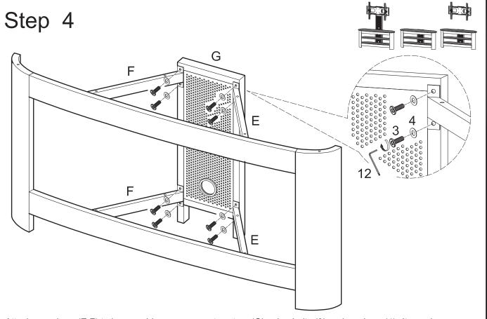
Attach crossbars (E,F) to lower cable management system (G) using bolts (3) and washers (4). *It may be necessary to slightly loosen the bolts from Step 3 in order to align crossbars (E,F) properly.* Tighten all bolts (3) with wrench (12).
