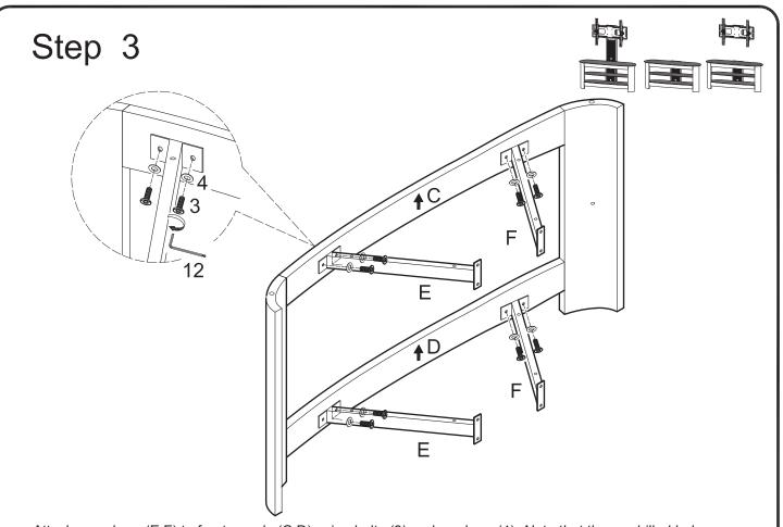
Attach crossbars (E,F) to front panels (C,D) using bolts (3) and washers (4). *Note that the predrilled holes on the lengths of crossbars (E,F) will face up.* Tighten bolts (3) with wrench (12).
