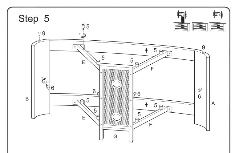
Screw suction cup pins (5) into crossbars (E,F). Screw pins (6) into legs (A,B) and lower cable management system (G). Insert rubber pads (9) into legs (A,B).
