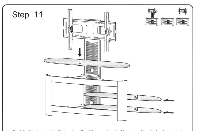
Carefully slide glass shelves (M) into place. Carefully place glass shelf (L) on top of the stand and gently push down to secure.
