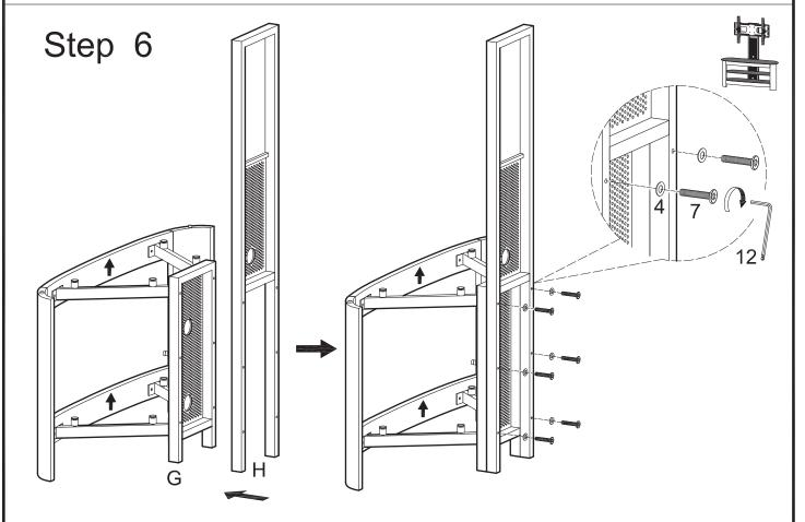
Attach upper cable management system (H) to lower cable management system (G) using bolts (7) and washers (4). Tighten bolts (7) with wrench (12).
