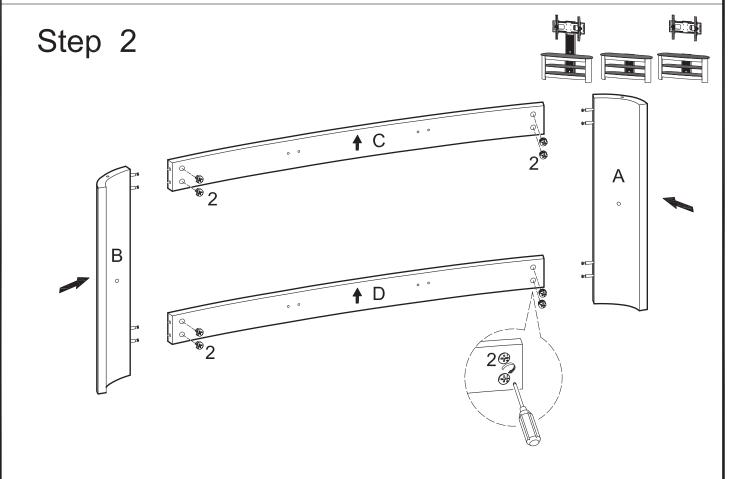
Insert cam locks (2) into front panels (C,D). Attach legs (A,B) to front panels (C,D) using cam bolts as guides. Tighten cam locks (2) with a screwdriver.
