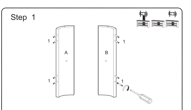
Screw cam bolts (1) into legs (A,B).
