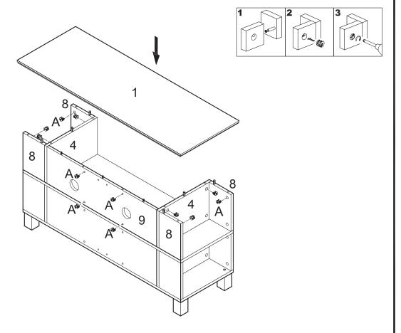
Insert large cam locks (A) into panels (4,8) and back panel (9). Attach stand top (1) to the stand assembly using cam bolts and dowels as guides. Tighten large cam locks (A) with a screwdriver.
