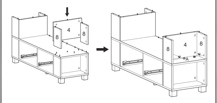
Attach the second set of panels (4,8) to the opposite end of the stand assembly using cam bolts and dowels as guides. Insert large cam locks (A) into panels (4,8) and tighten with a screwdriver.
