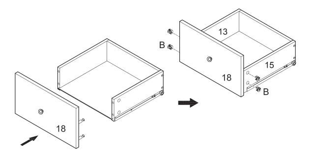
Attach drawer front (18) to the second drawer assembly using cam bolts as guides. Insert small cam locks (B) into drawer sides (13,15) and tighten with a screwdriver.
