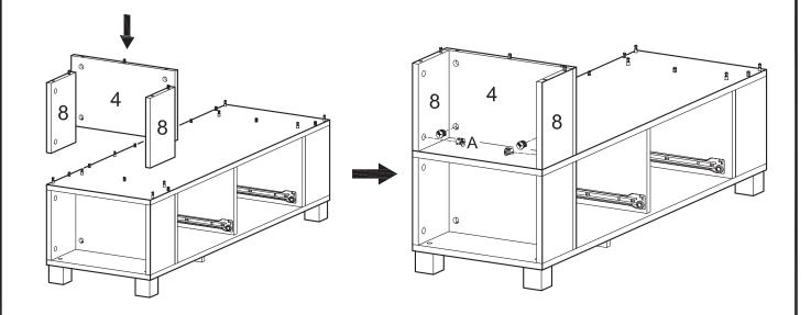
Attach panels (4,8) to the stand assembly using cam bolts and dowels as guides. Insert large cam locks (A) into panels (4,8) and tighten with a screwdriver.
