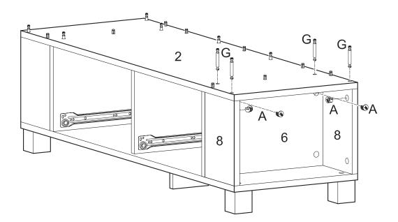
On opposite end of stand assembly, insert long cam bolts (G) into middle panel (2). Insert large cam locks (A) into panels (7,8) and tighten with a screwdriver.
