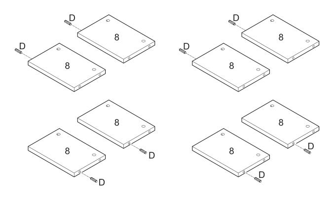
Insert short dowels (D) into panels (8) on appropriate sides.
