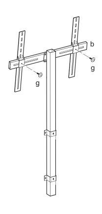
Slide mounting bars (c) onto lateral support bar (b). Secure mounting bars (c) by screwing adjustment knobs (g) into place.
