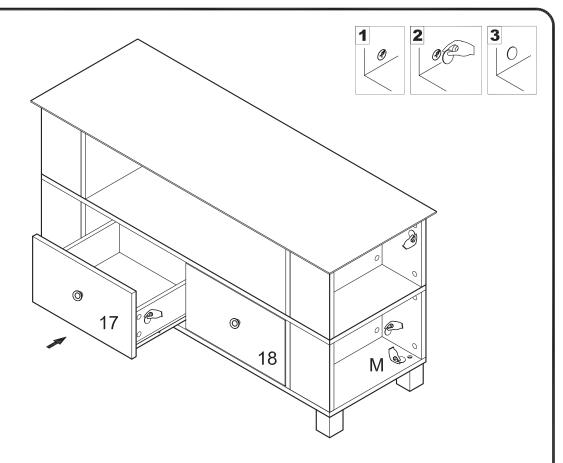
Carefully slide drawers into the stand assembly. Cover all visible cam locks with stickers (M) as desired.
