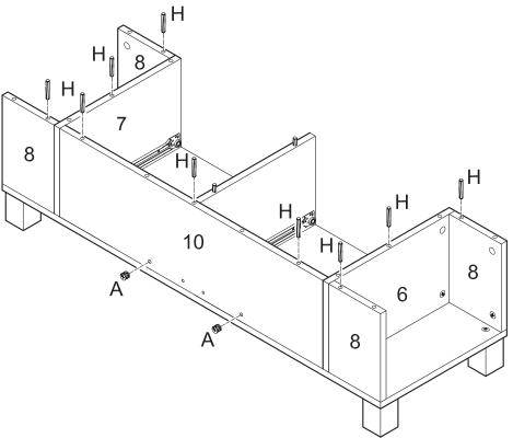
Insert cam locks (A) into back panel (10) and tighten with a screwdriver. Insert long dowels (H) into panels (6,7,8) and back panel (10).
