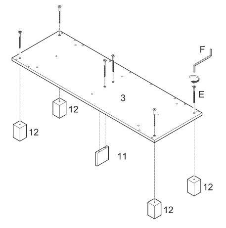
Attach feet (12) and stand support (11) to stand base (3) using large bolts (E) and wrench (F).
