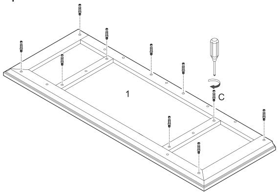
Screw short cam bolts (C) into stand top (1).
