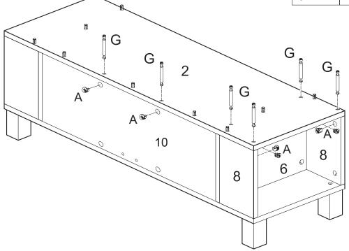
Insert long cam bolts (G) into middle panel (2). Insert large cam locks (A) into panels (6,8) and back panel (10). Tighten with a screwdriver to secure middle panel (2).
