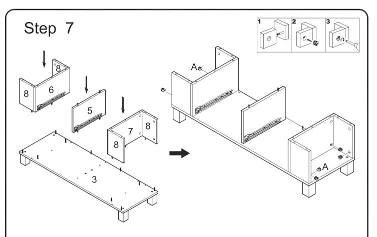
Attach panels (5,6,7,8) to stand base (3) using cam bolts and dowels as guides. *Note that panels (8) are not attached to panels (6,7), but that all panels should align when attached to stand base (3).* Secure panels (6,7,8) to stand base (3) by inserting large cam locks (A) into panels (6,7,8) and tightening with a screwdriver.
