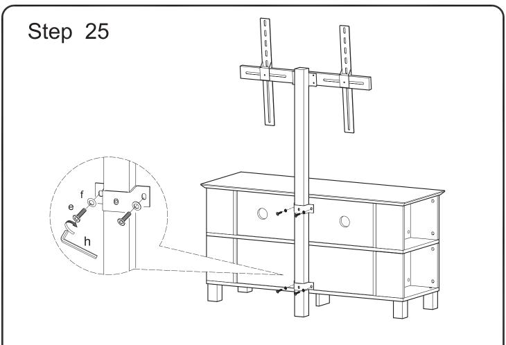
Attach TV mount to stand assembly using bolts (e) and washers (f). Tighten bolts (e) with wrench (h).
