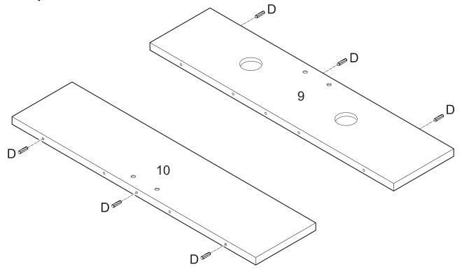
Insert short dowels (D) into back panels (9,10).
