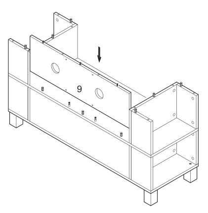
Carefully slide back panel (9) into place at the back of the stand assembly. Use cam bolts and dowels as guides.
