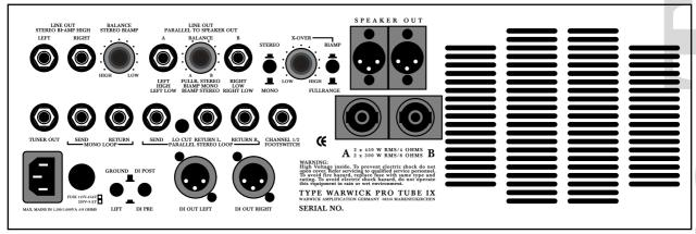
**GROUND LIFT** switch isolates the earth connection from the ground of signal. Should several devices be simultaneously connected to earth by the same conductor as well as via line connections, a so called hum loop might appear. In this case operate GROUND LIFT to eliminate the current hum.
