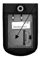
This battery does not have to be replaced until prompted by a warning message. If you see a transparent film insulating the backup battery, please remove it now.
