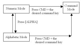
Press [ALPHA] to toggle between Numeric (block cursor) and Alphabetic (underscore cursor) entry modes. Characters are selected by quickly pressing a key one, two or three times.
