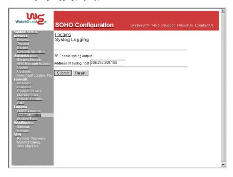
3 Enable the checkbox labeled **Enable syslog output**.
