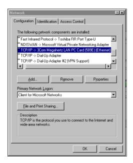
3 Scroll through the list of installed network components. Double-click the **TCP/IP** network component which is bound to your Ethernet card. Look for (Ethernet) in parentheses. The TCP/IP Properties dialog box appears.
