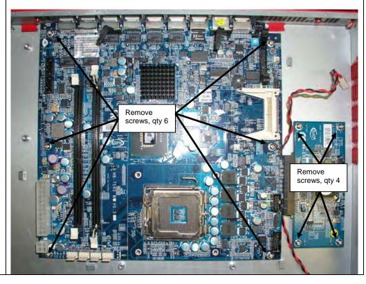
3.19 – Unplug the Ethernet ports on the motherboard from the chassis and unplug the Cavium card from the motherboard. Remove the motherboard and the Cavium card.
