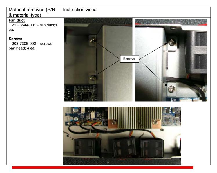
3.12 - Cut cable ties for fans, unplug fans from motherboard, and remove fans.
