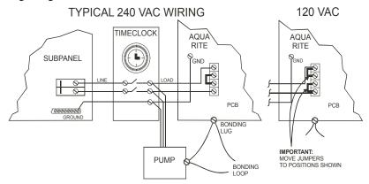
Note: Wire the pump directly to the timeclock--do not use the Aqua Rite as a junction box.
