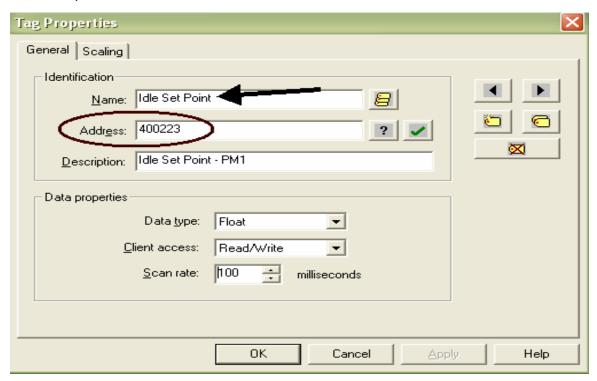
40. Now that the tags are created execute the OPC quick client as illustrated in step 33. Once running, click on the tag created to modify the assembly. In this case, "New Assembly - Pointer 12". Based on the "Description" field in the screen shot in step 38 and 39 pointer 12 will become the Idle Set Point of PM1 once changed. The value to be written below reflects this.
