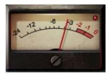
The PuigTecMEQ-5 meters display output level in dBFS. The LED located in the upper right corner lights up when output signal is clipping.
