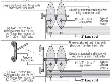
**For Center Hinges**, align the slots of the lower hinge leaf with the pre-drilled holes or at each center stile at the top rail of bottom section. Using the center hinge as a template, drill pilot holes, 1" deep into the bottom section with a 1/8" drill bit (if needed).
