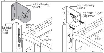
Position the left hand end bearing bracket up against the jamb and the horizontal track, as shown. Fasten the left hand end bearing bracket to the horizontal track with (1) 3/8"-16 x 3/4" truss head bolt and (1) 3/8"-16 nut. Secure the left hand end bearing bracket to the jamb using (3) 5/16" x 1-5/8" lag screws. Repeat same process for the other side.
