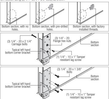
Next, secure the bottom corner bracket to the bottom section using (1) 1/4"-14 x 1" tamper proof screw to the left hand bottom corner bracket, as shown.
