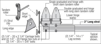
For Center Hinges, align the slots of the lower hinge leaf with the pre-drilled holes or at each center stile at the top rail of bottom section. Using the center hinge as a template, drill pilot holes, 1" deep into the bottom section with a 1/8" drill bit (if needed).
