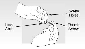
Insert middle Meat Clamp Arm into top into top of the Lock Arm as shown. Tighten top Thumb Screw to lock Meat Clamp into shaft.
