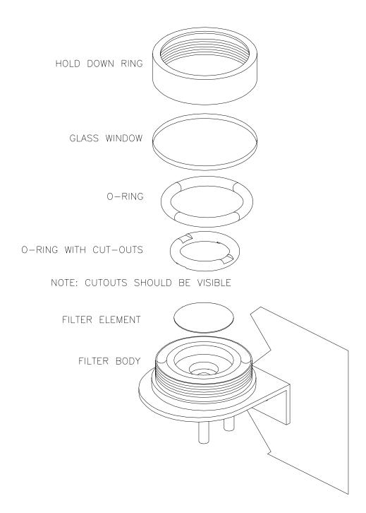
Figure 5.1 - Replacing the Particulate Filter
