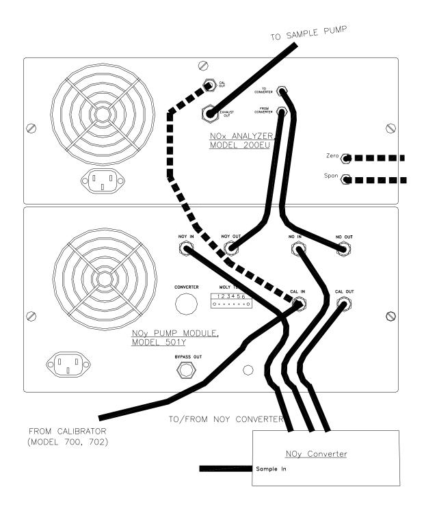
**Figure 1.1 - Rear Panel Pneumatic Connections**
