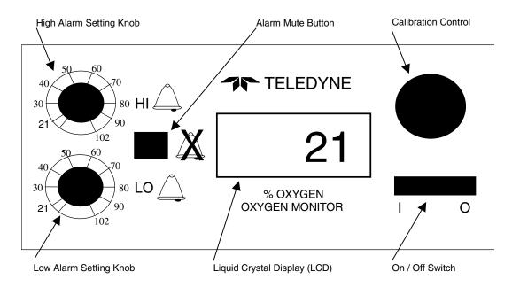
On / Off Switch Allows the operator to turn the instrument on and off.
