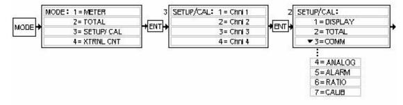
Pressing the **MODE** key causes the **MODE** menu to be displayed. Choose the **SETUP/CAL** mode by pressing the number "3" key then **ENTER**. A **CHANNEL SELECT** menu is presented on the display. It should be noted that, although the user must select a specific channel number, some choices in the following menus may affect the operation of all channels and/or the display (ex; Display Brightness, type of communication). See the following menu options for more details.
