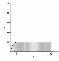
Each channel samples the incoming signal at a rate corresponding to the preset A/D conversion rate in Hz. At each sampling interval, the TOTALIZER function multiplies the average signal, as a fraction of the full-scale value (5v, 10v or 20 mA), times the *span*, or *cal*, value. This results in a rate for that interval. Next, a time element factor is determined according to the flow rate programmed for that channel as follows.
