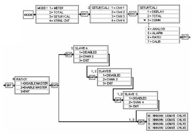
Press the **MODE** key and then **3 + ENTER**. Select channel one by pressing **1 + ENTER**. Choose **RATIO** by pressing the **6** key **+ ENTER**. Channel one (1) is enabled as the master when you press **2 + ENTER**.
