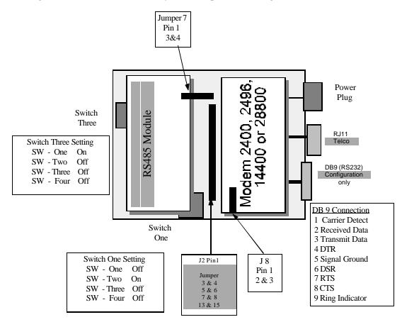
Final Factory Configuration (MIUXXXX/485) for PEXXX modem module No, Power saving modes, No Auto Reset mode Switch two ON Switch one, three and four are OFF.
