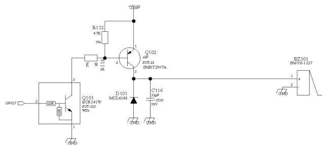
A sample interface scheme is included below to give you an idea of how to interface a Buzzer to the GPIO7:
