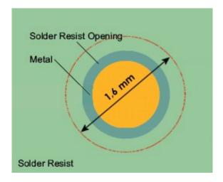
Holes in pad are allowed only for blind holes and not for through holes.
