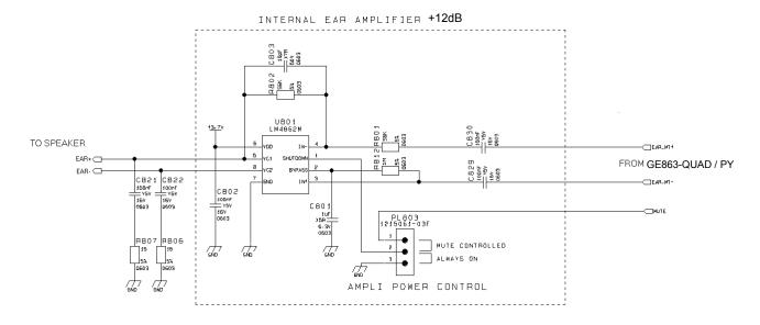
Some amplifier require a low impedance load at high frequency in order to avoid auto oscillation, this can be made with a capacitor (100nF) in series with a resistor  $(15\Omega)$ .
