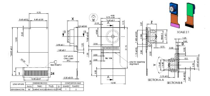
Fig 2. Camera Socket Connector
