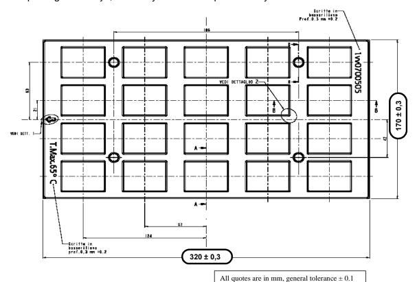
Note that trays can withstand a maximum temperature of 65° C.
