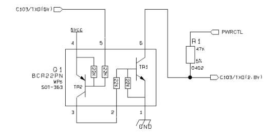
NOTE: The UART input line TXD (rx\_uart) of the GE863-QUAD/PY is NOT internally pulled up with a resistor, so there may be the need to place an external 47KΩ pull-up resistor, either the DTR (dtr\_uart) and RTS (rts\_uart) input lines are not pulled up internally, so an external pull-up resistor of 47KΩ may be required.
