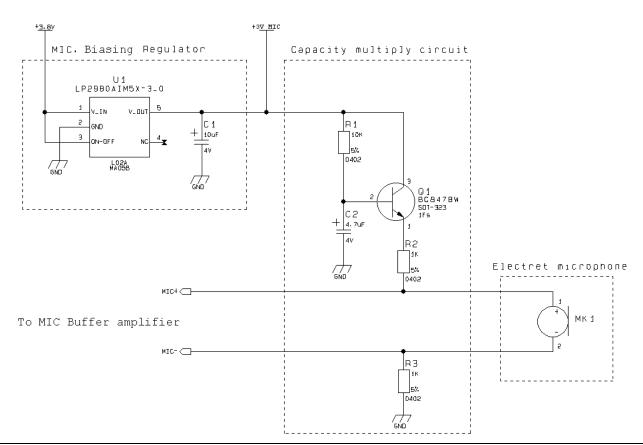
NOTE: In the balanced application the resistors R2 and R3 must have the same value to keep the circuit balanced.
