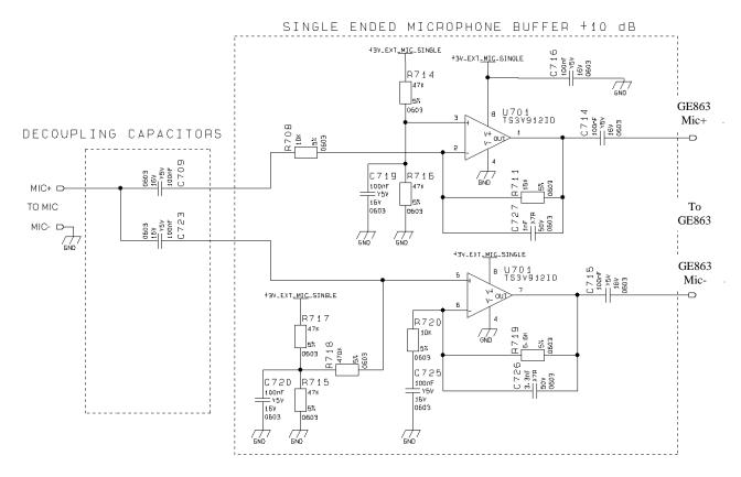
The above schematic can be used for a single ended (*buffered unbalanced*) microphone; the required biasing circuitry is not included. Note also that the capacitor C3 is not needed. The gains of the two amplifiers are given by the formulas:
