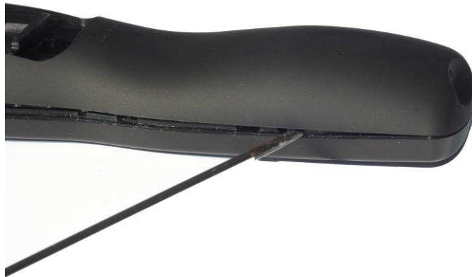
Figure 15: Opening the remote control, step two
