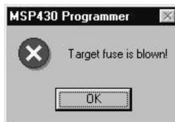
Figure 2–3. Communication Error Box for Blown Fuse
