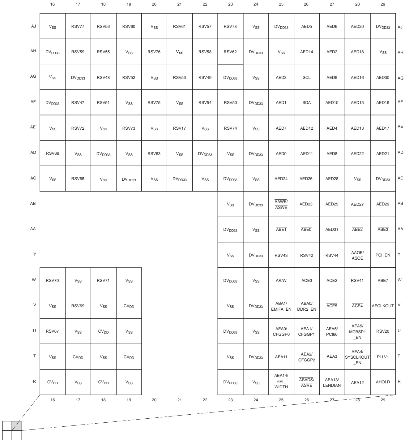
Figure 2-3. C6454 Pin Map (Bottom View) [Quadrant B]
