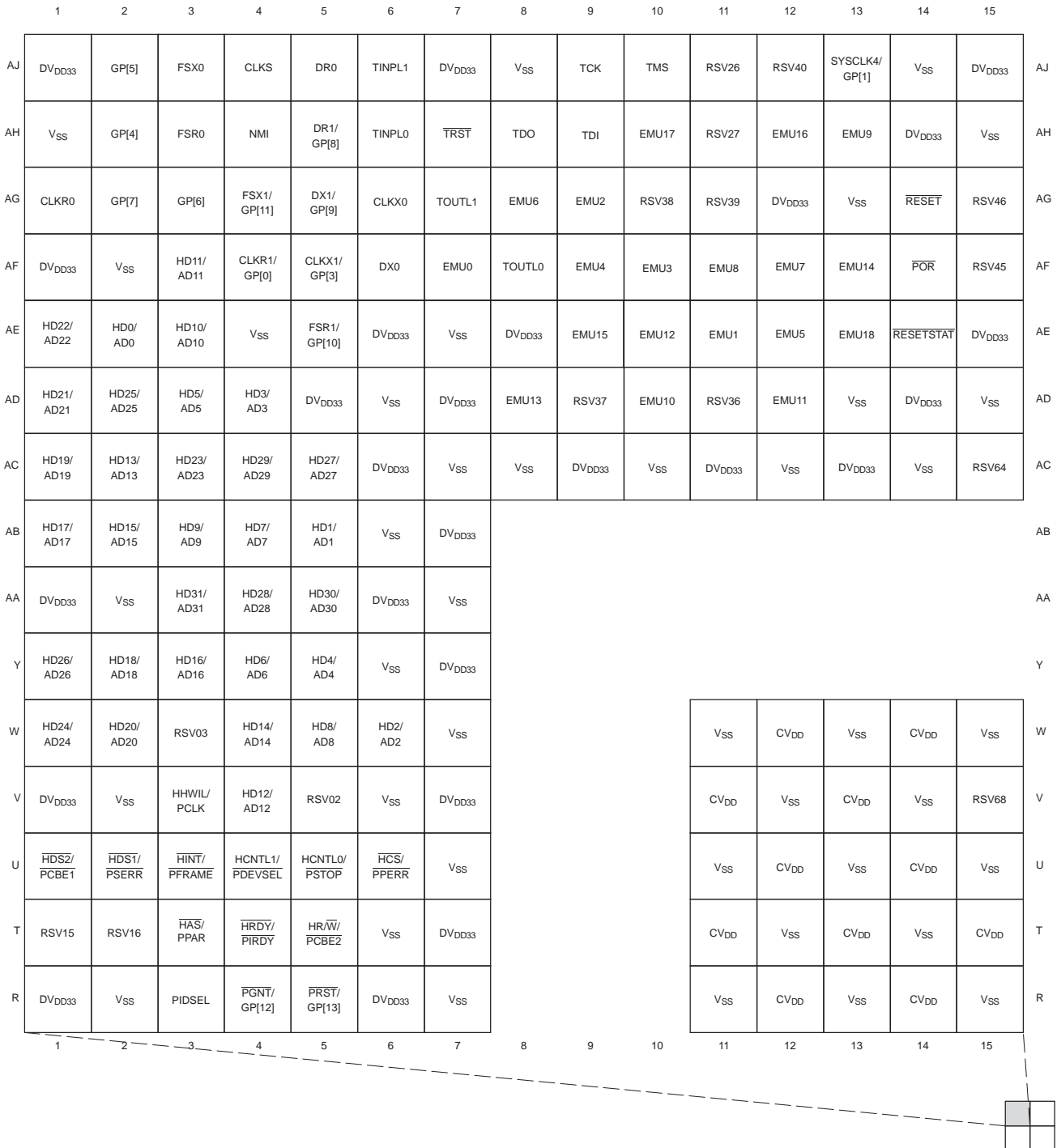
Figure 2-2. C6454 Pin Map (Bottom View) [Quadrant A]
