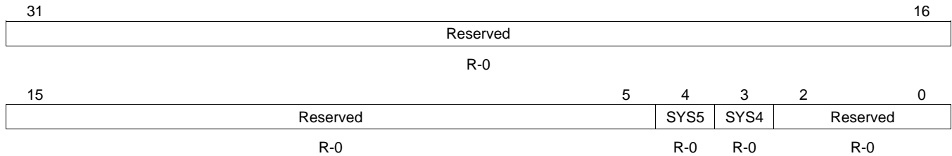
Figure 7-19. PLLDIV Divider Ratio Change Status Register (DCHANGE) [Hex Address: 029A 0144]
