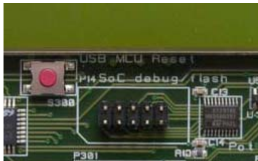
Figure 5: SmartRF04EB debug connector for debugging CC2511 Dongle / other external target systems
