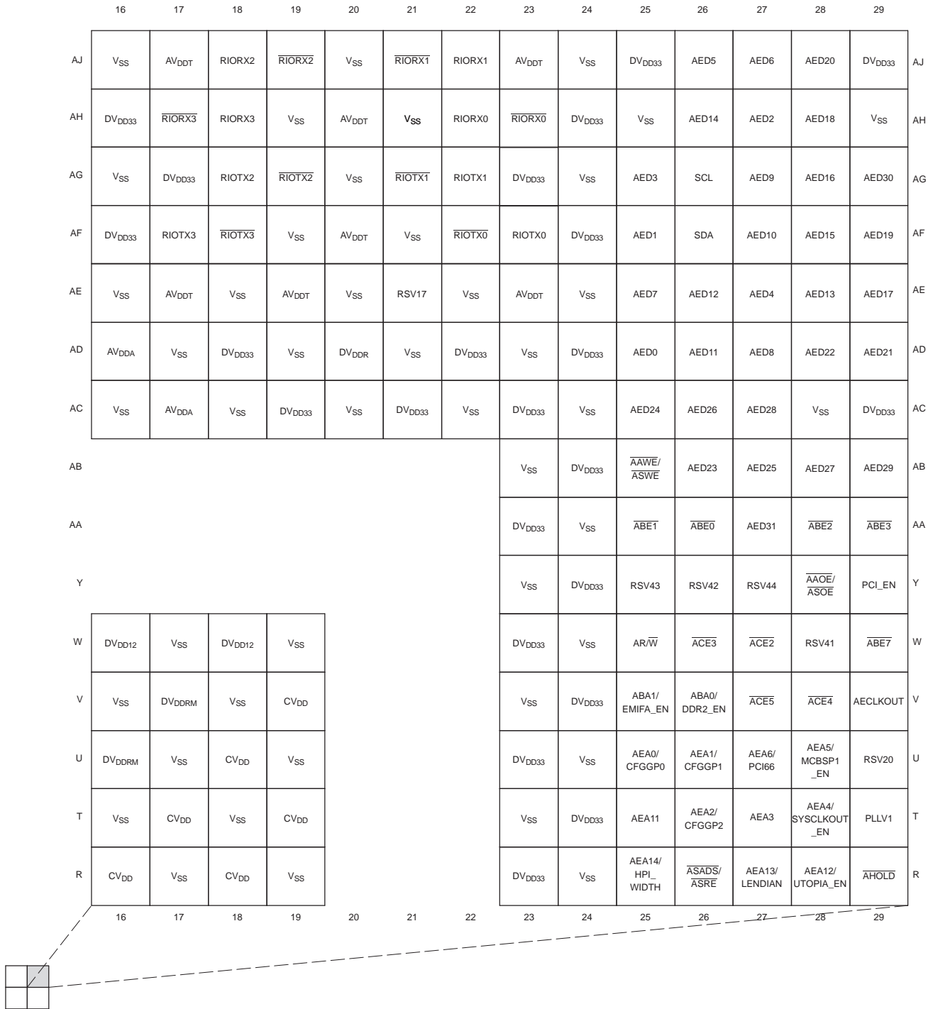
Figure 2-3. C6455 Pin Map (Bottom View) [Quadrant B]
