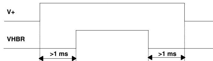
Figure 3–1. Recommended Power-Up and Power-Down Sequence
