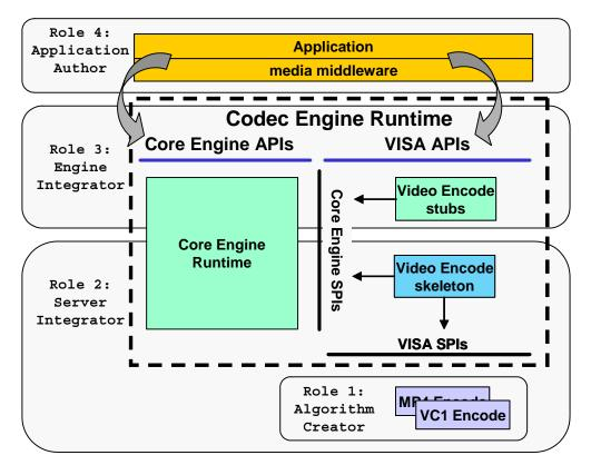
The application (or middleware it uses) calls the core Engine APIs and the VISA APIs. The VISA APIs use stubs to access the core engine SPIs (System Programming Interfaces) and the skeletons. The skeletons access the core engine SPIs and the VISA SPIs. The VISA SPIs access the underlying algorithms.
