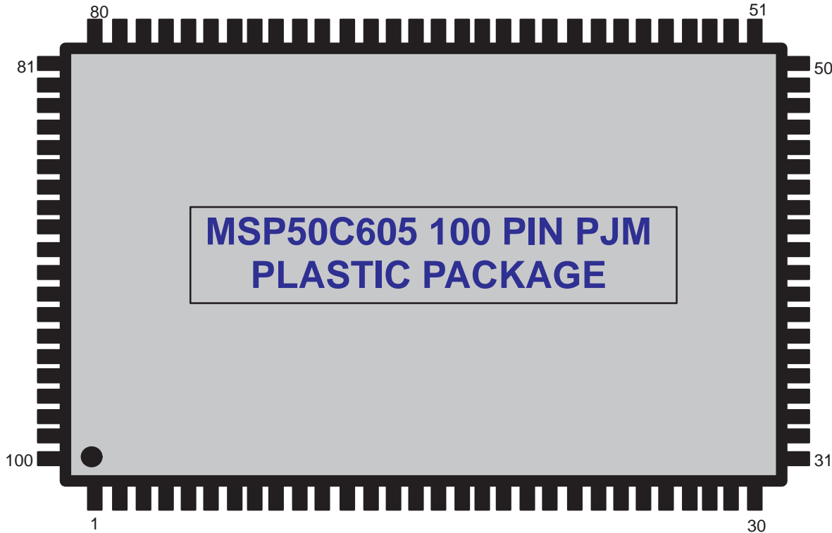
Figure A-3. MSP50C605 100-Pin PJM Package
