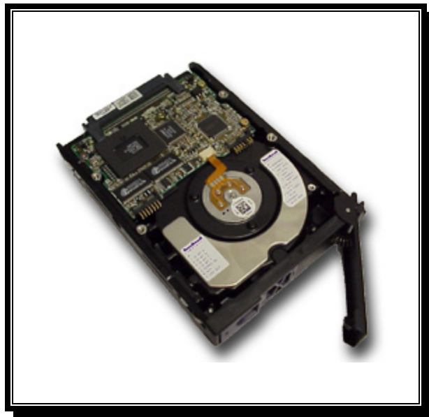
Figure B-6 TDD21 18 gigabyte replacement hard drive
