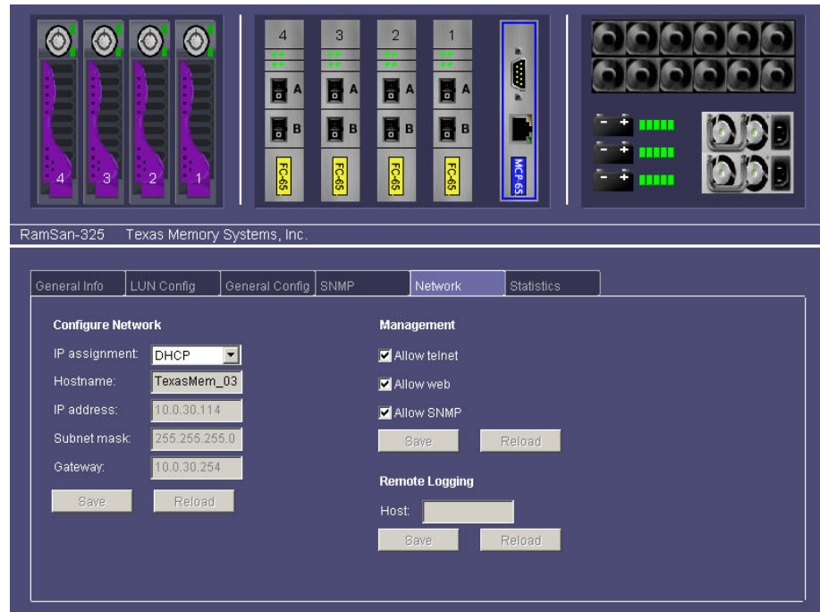
Figure 4-7: Web Management Ethernet Configuration
