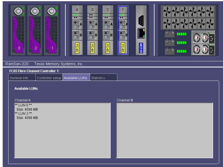
Figure 6-6: Viewing LUNs Assigned to FC ports via Web Interface
