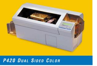
The P420's rugged, all metal enclosure houses a lowmaintenance print mechanism that includes self-cleaning card handling, high capacity ribbon system, two-line LCD control panel, and convenient card reject hopper. The reject hopper separates cards that fail encoding prior to printing, saving valuable printer ribbon. The enclosure includes a viewing window to monitor the printing process without opening the unit. Transparent input and output hoppers provide visual card capacity status.
