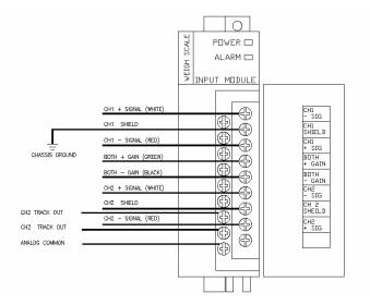
To ensure proper operation and high immunity to electrical noise, always use Helm strain gage cable.
