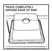
1. If it is necessary to cut out the counter top, invert sink and position onto the counter top. Locate sink front to rear and so that the bowl will not interfere with the cabinets below. Trace a pencil line around the outside edge of the sink and remove the sink from the counter top.
