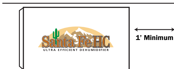
Figure 3: Installation requires a minimum 1' exhaust clearance.
