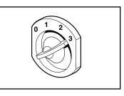
The blower speed control knob is located on the right front of the intake. The intake must be raised in order to use the control knob. There are four blower speed settings represented by numbers "0" (Off), "I" (Low), "2" (Medium), and "3" (High).
