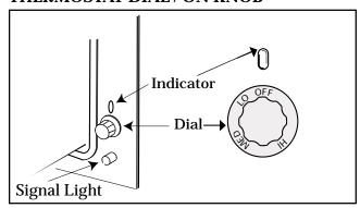
Open the drawer. The thermostat dial is on the right side of the front frame.
