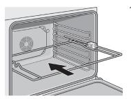
1. Insert rotisserie rack half way into the oven on rack position 4.
