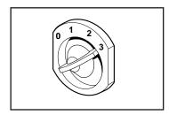
The blower speed control knob is located on the right front of the intake. The intake must be raised in order to use the control knob. There are four blower speed settings represented by numbers "0" (Off), "I" (Low), "2" (Medium), and "3" (High).
