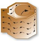
heat exchanger is fabricated out of 13-gauge copper coated steel. Some manufacturers use less expensive, thinner 14 or 16-gauge steel. Thermo Pride's copper powder coating helps prevent cor-
