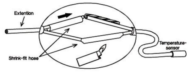
Slide larger tubing (about ¾ ") over the entire completed splice. Heat gently all around until tubing shrinks tight. This connection can then be drawn gently into the pipe work. Only two of the wires are required for the sensor cable; the other two wires are spare wires.
